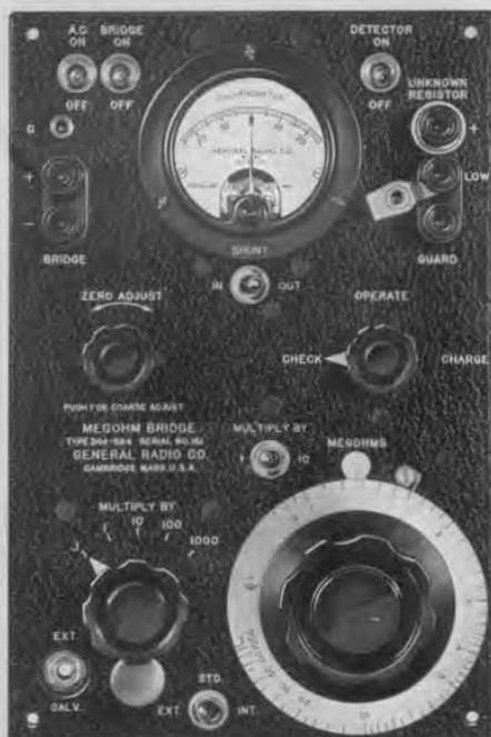
FIGURE 3. Panel view of a TYPE 544-BS4 Megohm Bridge. In addition to the switches shown, two others can be installed: a charge-discharge switch and a polarity reversing switch.
